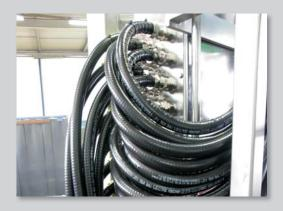
**Anti-Static performance:** Surface resistance < 10<sup>9</sup> Ohm, meeting the requirements of standard NEN-EN-IEC 60079-0, section 26-13.
